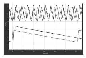
Figure 8. Comparison of static and dynamic hysteresis.
