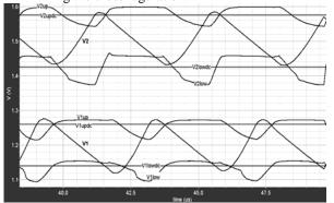
Figure 6. Steady state  $V_1$  and  $V_2$  when load currents  $I_1=I_2=300$  mA.
