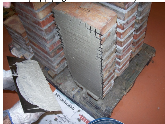
d) Applying the final mortar layer
