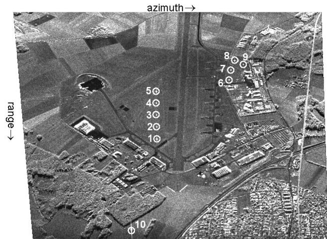
Fig. 1. Reflectivity image of the Oberpfaffenhofen test site with the position of all ten CRs marked and numbered in white (image in zero-Doppler geometry, processing squint =  $3^\circ$ ).
