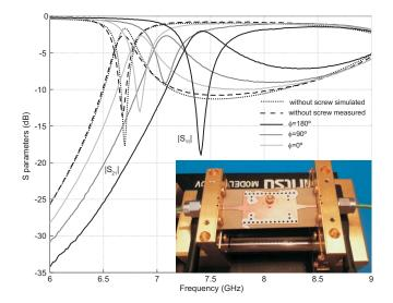
Fig. 5. Measured results of the prototype. The inset shows the picture of the fabricated prototype.
