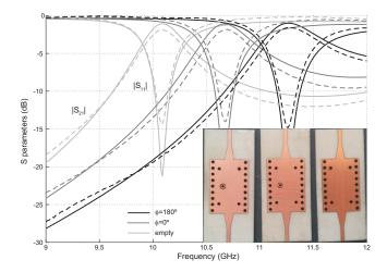
Fig. 3. Measured (solid) and simulated (dashed) scattering parameters for a cavity with a tuning element placed at x = 2mm, and picture of the fabricated resonators (inset).
