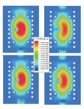
Fig. 2. Electric field at the resonant frequency for the cavity with full slot *a*), with contact for  $\phi = 0$  *b*), without slot *c*), and with contact for  $\phi = 180$  *d*).
