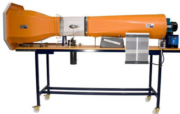
Figura 7.2 Túnel aerodinàmic Armfield C2. [www.discoverarmfield.com]
