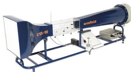
Figura 7.1 Túnel aerodinàmic Armfield C15-10. [www.discoverarmfield.com]
