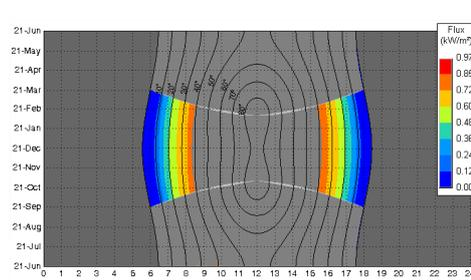
**Fig. 10** Isochronous projection of solar radiation flux during one year
