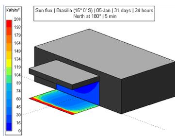
**Fig. 8** Solar radiation on floor and wall from Dec. to Jan.
