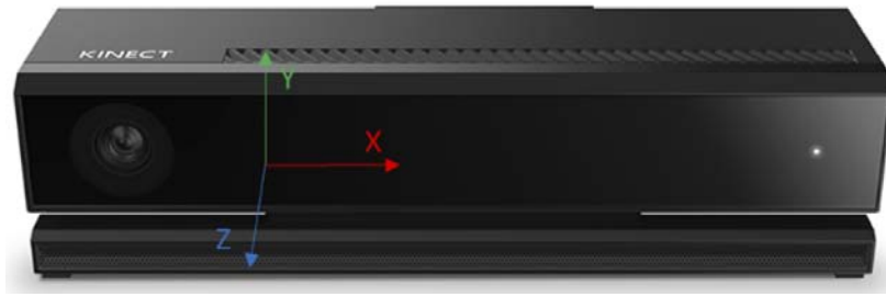
Figure 30: The Kinect camera space coordinate system
