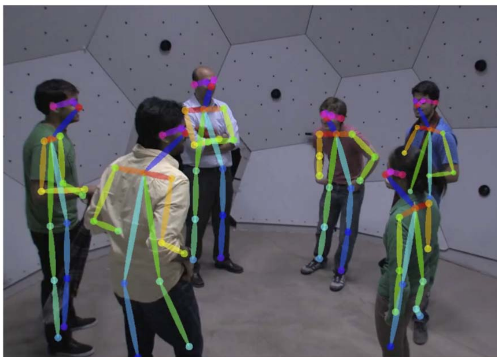
Figure 20: Multi-person pose estimation with OpenPose [7]
