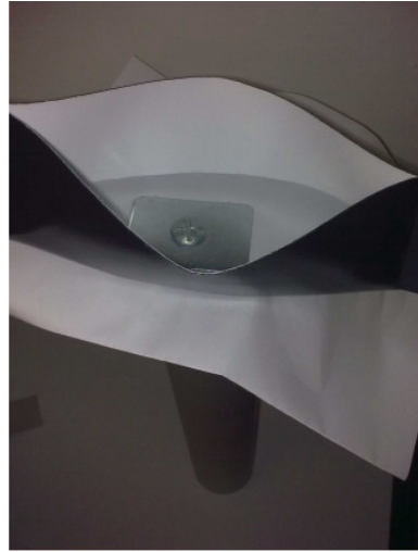
Figure 11 : Tensile insulation support : large prototype and water tightness testing of the bolts
