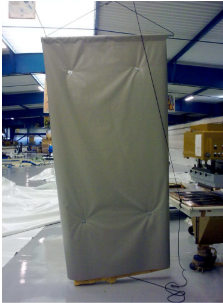
Figure 11 : Tensile insulation support : large prototype and water tightness testing of the bolts
