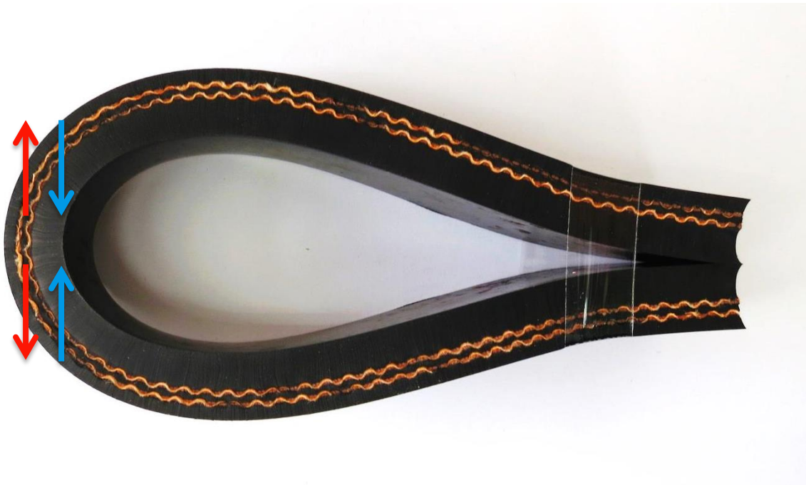
Figure 4: Bending characteristics of membranes for inflatable dams
