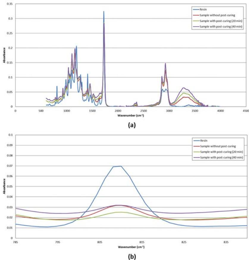
Fig. 8. (a) Results obtained from FTIR spectrometry; (b) Detail of the absorption band (810 cm<sup>-1</sup>) where the photoconversion ratio is calculated.
