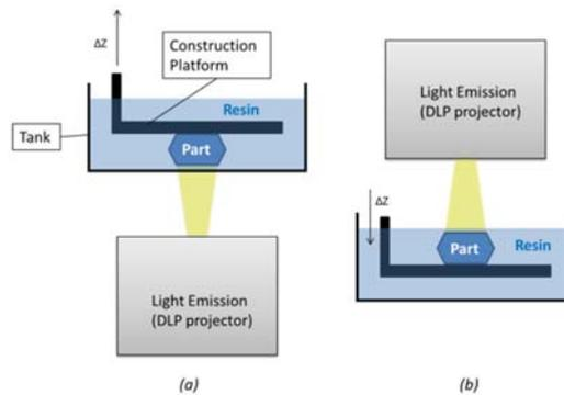
Fig. 4. (a) Bottom-up; (b) Top-down DLP schematics.
