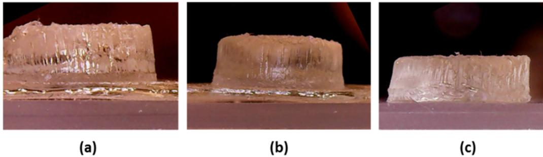
Fig. 1. Experimental solidified samples obtained after different exposure doses (a) 780 mJ/cm<sup>2</sup>; b) 624 mJ/cm<sup>2</sup>; c) 468 mJ/cm<sup>2</sup>.
