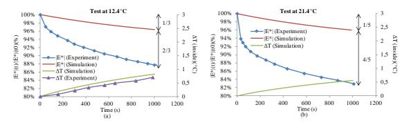
Figure 5: Normalized mixture complex modulus variation and temperature evolution: (a) test temperature: 12.4°C; (b) test temperature: 21.4°C
