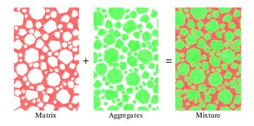
Figure 2: Biphasic Matrix/Aggregate cross-section mesh
