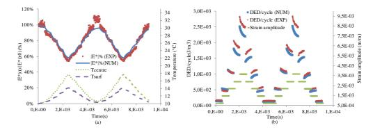
Figure 4: First up-and-down strain sweep test performed on B40/50 -Complex modulus and dissipated energy density data
