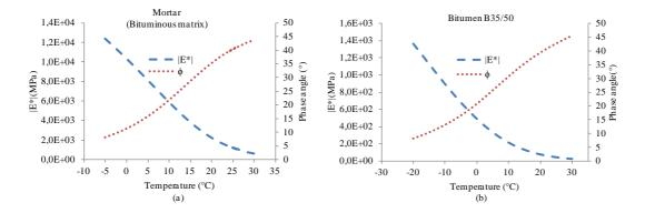
Figure 3: Modulus and phase angle master curves of bitumen and mortar at 10 Hz
