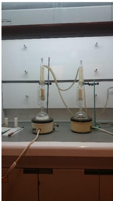
Figure 2.3.3: Soxhlet Extraction to measure sol fraction
