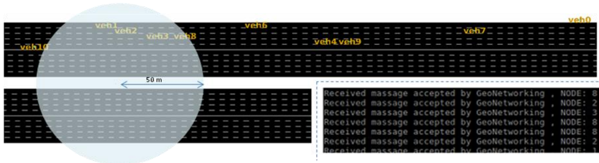
Fig. 31 - GeoNetworking situation: veh1, veh2, veh3 and veh8 inside, the others outside.
