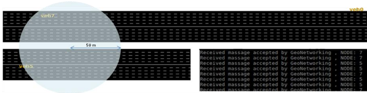
Fig. 32 - GeoNetworking situation: veh5 and veh7 inside, the others outside.
