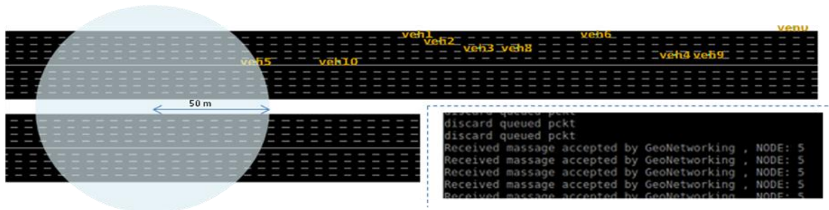
Fig. 29 - GeoNetworking situation: veh5 inside, the others outside.
