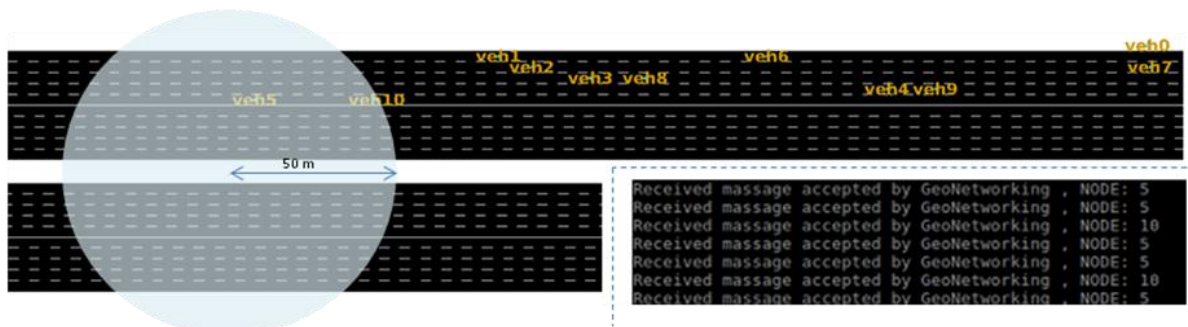
Fig. 30 - GeoNetworking situation: veh5 and veh10 inside, the others outside.
