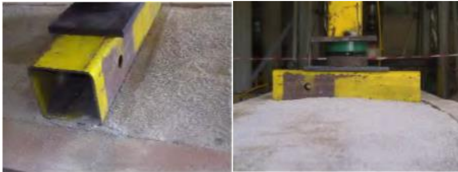
Figure 3-26 cave-in of the loading system (Serna, J., 2001).
