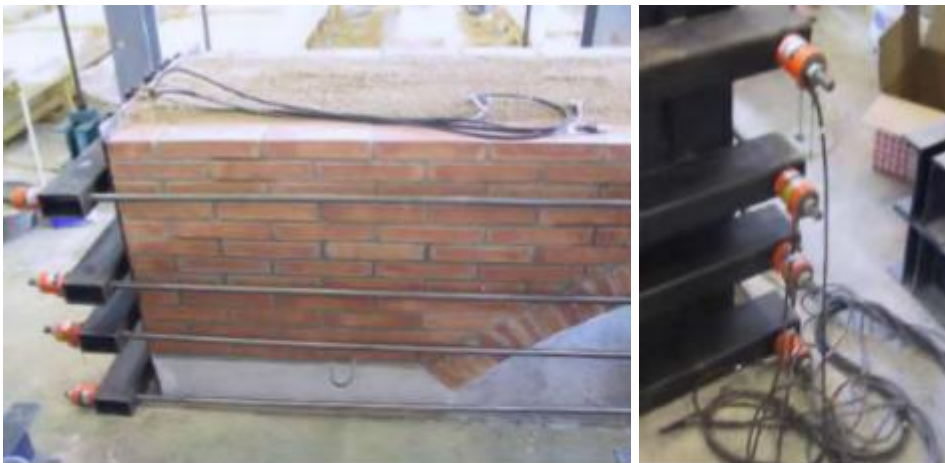
Figure 3-11 loading cells at the ties (Serna, J., 2001).
