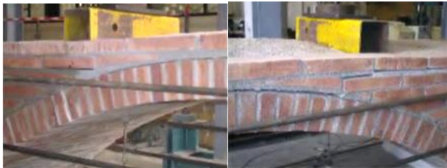
Figure 3-23 view of the plastic hinge under the loading point from both sides (Serna, J., 2001).
