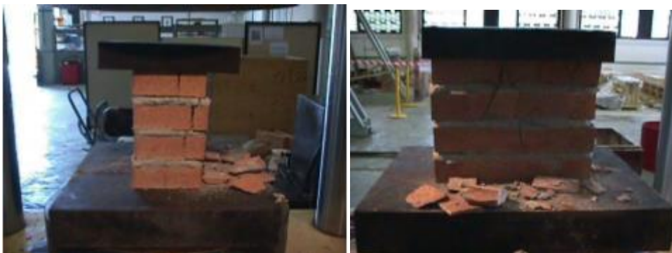
Figure 3-2 compression test of the masonry (Serna, J., 2001).
