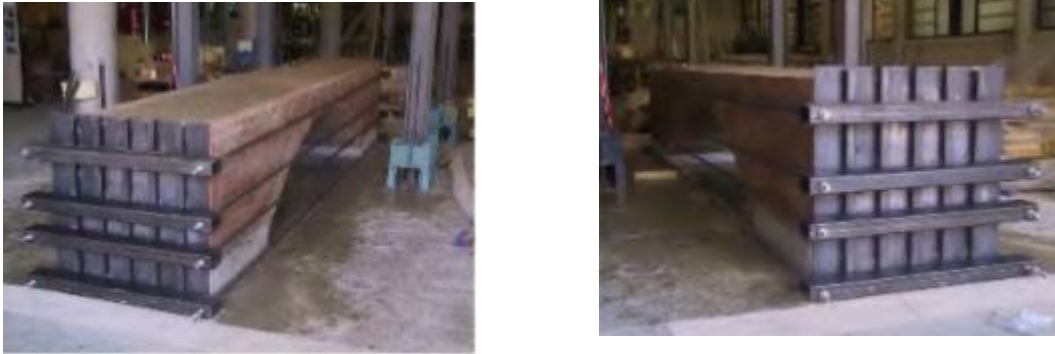
Figure 3-10 constructed bridge ready for the loading test (Serna, J., 2001).
