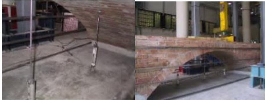
Figure 3-12 extensometers located under the arch (Serna, J., 2001).
