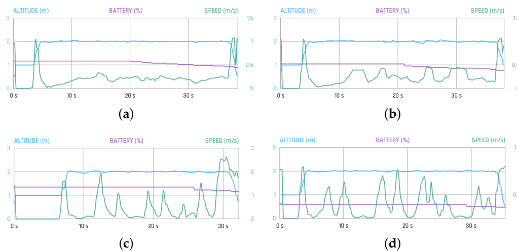
Figure 23. Results of two fixed obstacles for four different controllers. (a) Autonomous control; (b) bang-bang control (c) teleoperator with experience; (d) teleoperator without experience
