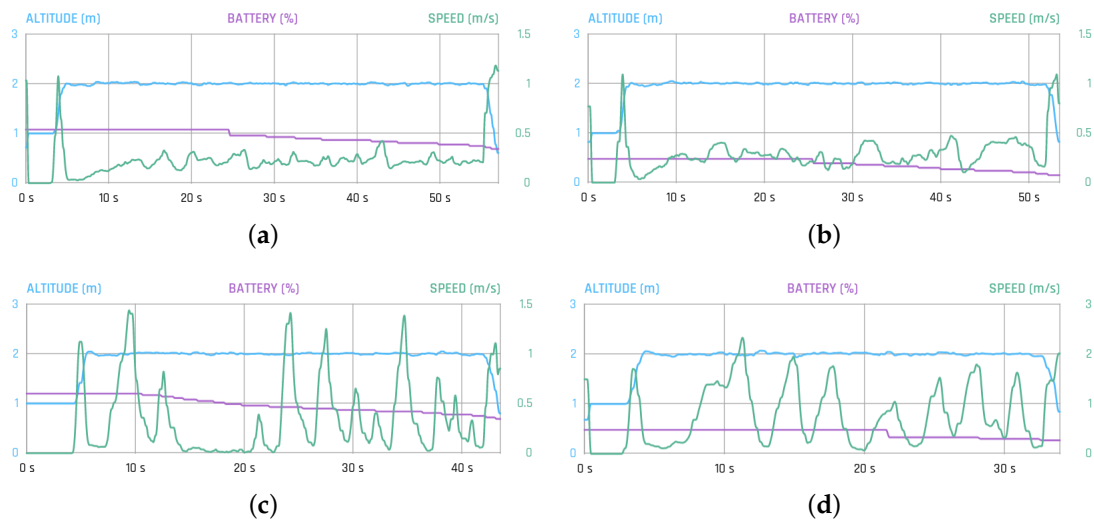
Figure 24. Results of three fixed obstacles. (a) Autonomous control; (b) bang-bang control (c) teleoperator with experience; (d) teleoperator without experience
