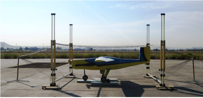
Fig. 5. Direct current injection test setup using coaxial return of SIVA UAV in INTA OATS.
