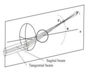
Figure 1. Oblique astigmatism in an off-axis object point for the lens-eye system; the different behavior in the sagital and tangential planes induces two different foci, creating oblique astigmatism
