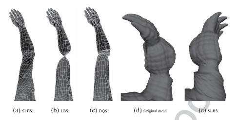
Figure 11. Deformation over an arm for two meshes performed by different deformation methods, with a 180° rotation. SLBS, segmentation-based linear blend skinning; LBS, linear blend skinning; DOS, dual quaternion skinning.
