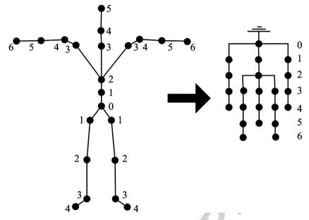
Figure 1. Equivalence between a logic skeleton used in animation and a n-ary hierarchy tree.
