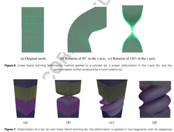
**Figure 7.** Detormation of a bar (a) with linear blend skinning (b), the deformation is applied in two segments with its respective loss of volume produced by a twist rotation greater than 180°. In our approach, we apply the deformation solely in one segment, preventing the loss of volume and self intersection (c) and (d).
