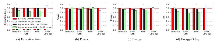
Fig. 10: Normalized execution time, power, energy, and energy-delay (ED) product for different CMP configurations and averaged per benchmark suite. We analyse only cores and L2 caches since the rest of CMP is shared and same for all configurations. Asymmetric++ CMP has the same area budget as Baseline CMP.
