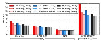
Fig. 7: BTB MPKI for different number of entries and associativity. We use branch address to index BTB.
