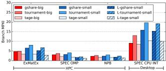
Fig. 5: Branch MPKI for different branch predictor configurations and benchmark suites.
