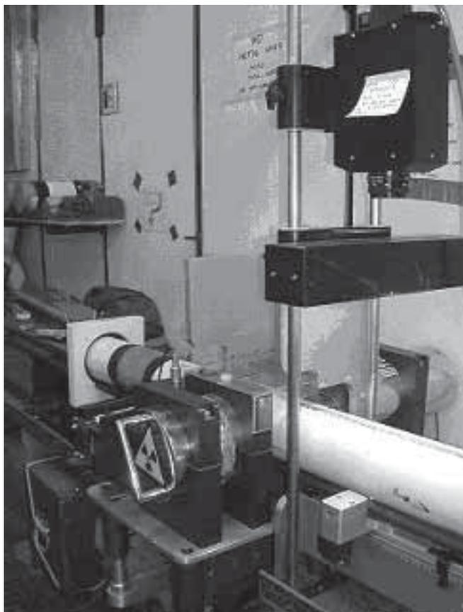
**Figure 1: Multi-Sensor Core Logger of the Oregon State University, installed onboard the R/V Roger Revelle, showing the Gamma-Ray, electrical resistivity and Magnetic Susceptibility sensors. Also, a visible-image camera-scan device is shown.**
