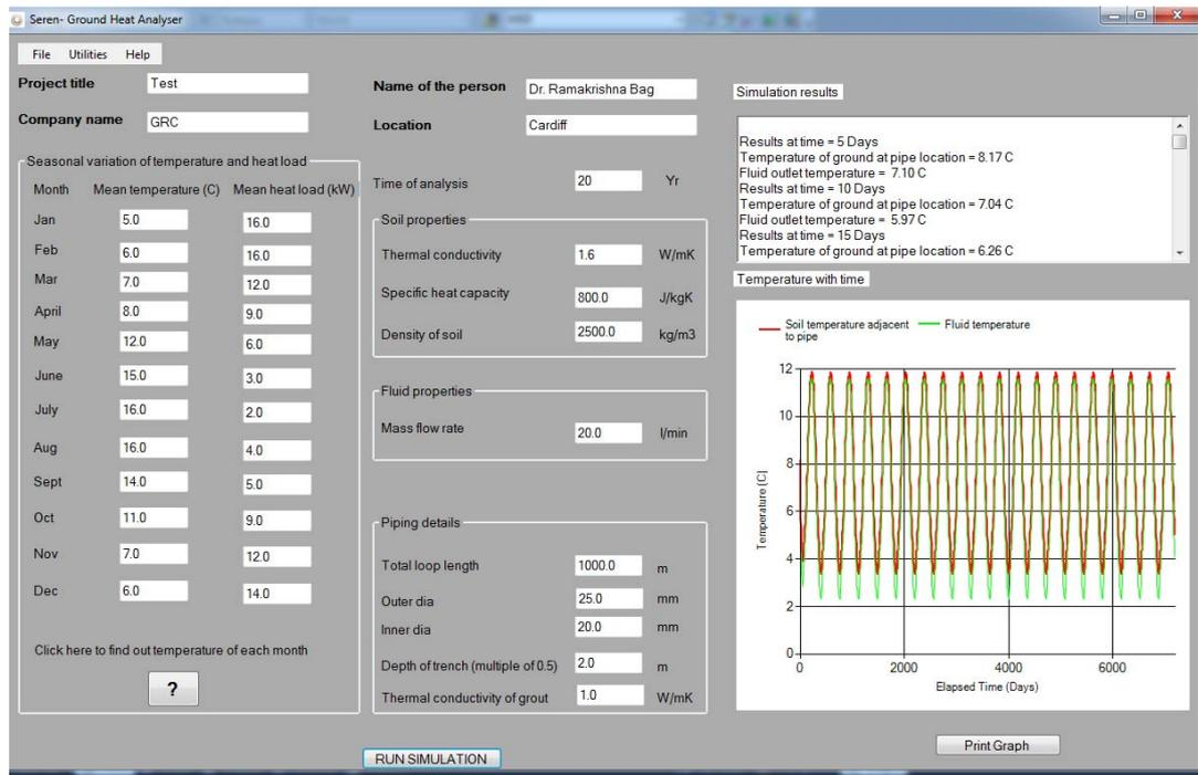
Fig.1: User interface of the numerical tool called “Ground Loop Analyser”.
