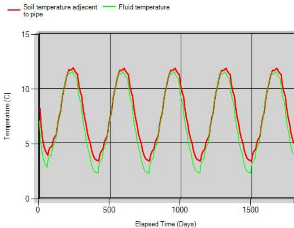
Fig. 3: Fluid outlet temperature and ground temperature obtained from numerical simulation using Ground Loop Analyser.
