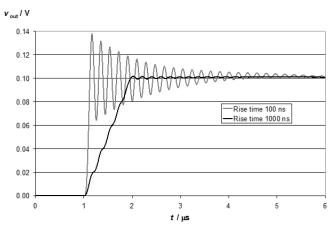
Output voltage when a 100 mV pulse has been applied
