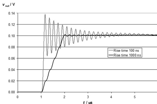
Output voltage when a 100 mV pulse has been applied
