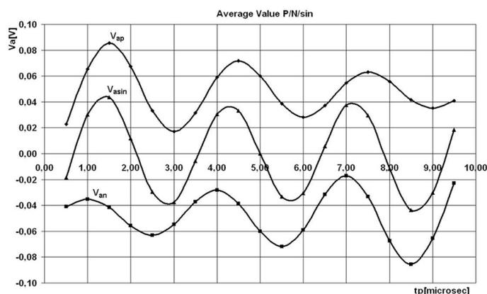
The average values of the oscillations:  $V_{ap}$ , during the positive pulse,  $V_{an}$ , during the zero level and their sum  $V_{asin}$
