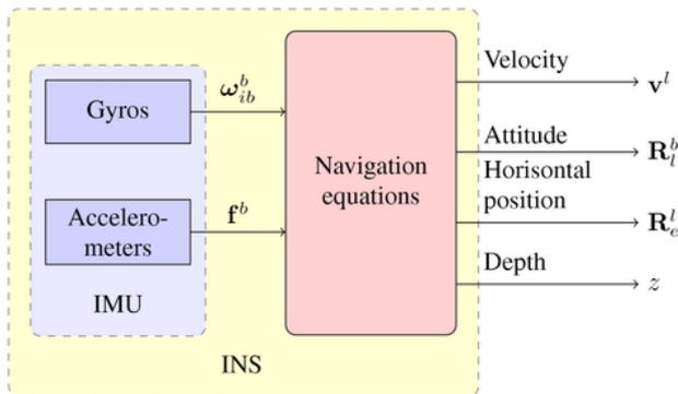
**Figure 1. A block diagram of an inertial navigation system (INS)**
