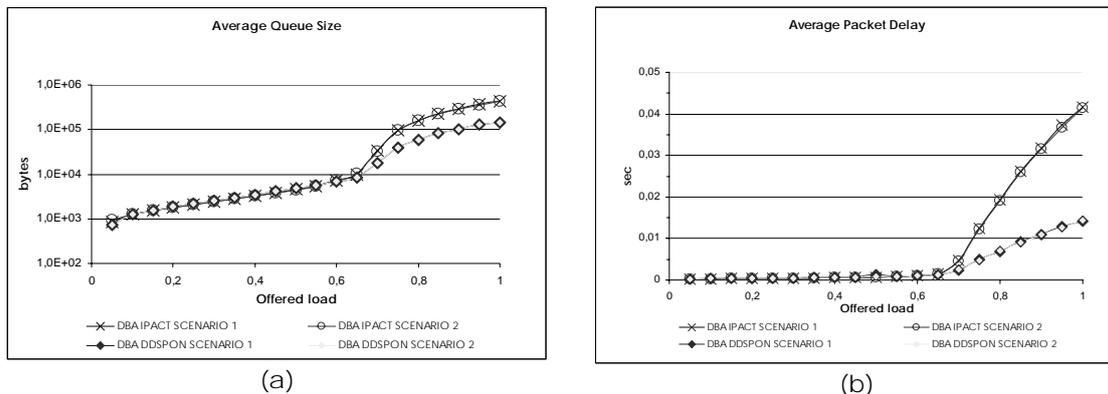
Figure 27. Average queue size and Average packet delay as function of offered load
