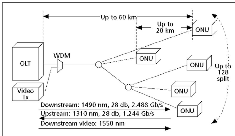
Figure 3. GPON physical network architecture
