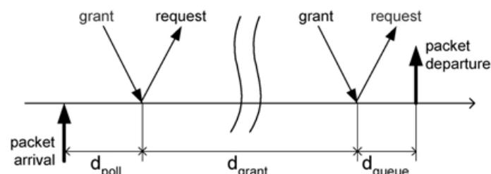
Figure 26. Components of packet delay
