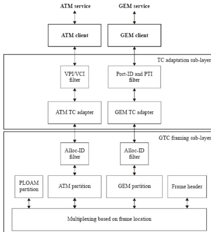
Figure 5. G.984.3 – Protocol stack for U-Plane and identification by partition and Port-ID or VPI
