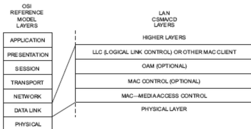
Figure 8. IEEE 802.3ah OAM sublayer relationship to the ISO/IEC Open Systems Interconnection (OSI) reference model and the IEEE 802.3 CSMA/CD LAN model
