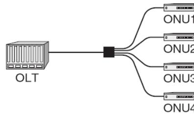
Figure 1. Passive Optical Network (Tree Topology)
