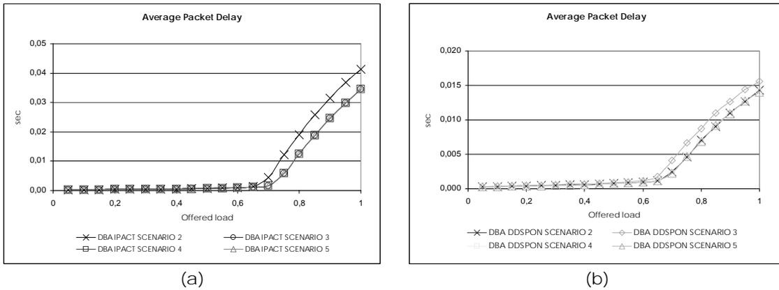
Figure 29. Average packet delay as function of offered load
