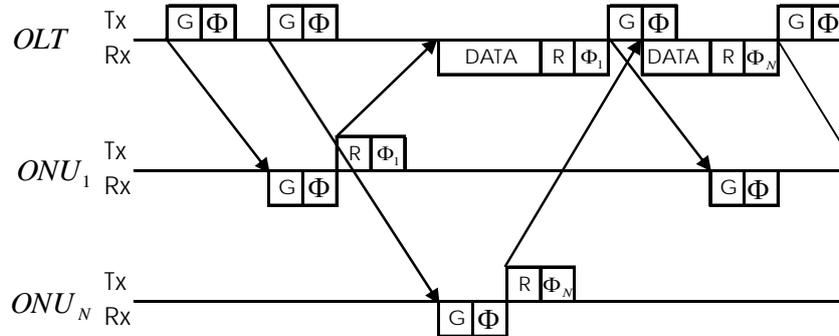
Figure 24. Illustration of the Interleaved Polling Mechanism
