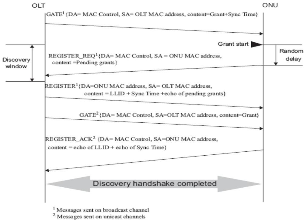
Figure 7. IEEE 802.3ah Discovery Handshake Message Exchange
