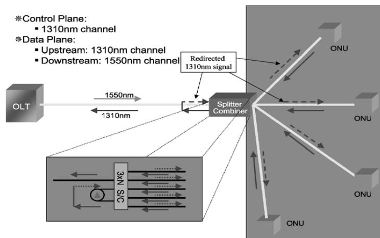
Figure 21. Proposed distributed EPON architecture
