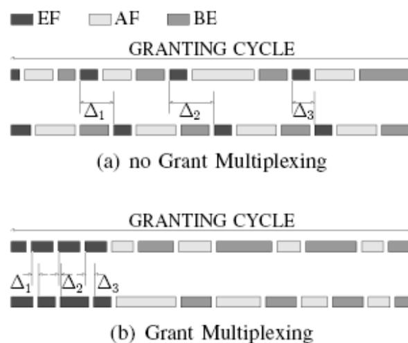
Figure 13. Bandwidth assignment with and without Grant Multiplexing
