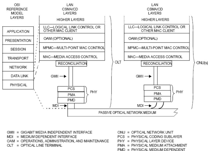
Figure 6. IEEE 802.3ah Architectural positioning of EFM: P2MP Topologies
