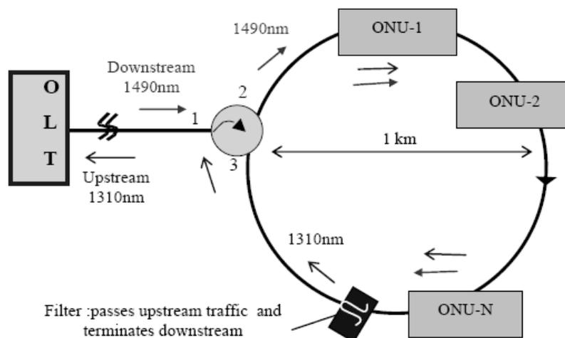
Figure 19. Ring-based EPON architecture
