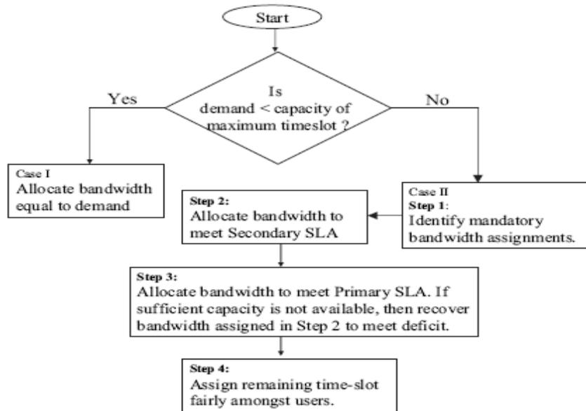
Figure 14. Flowchart for Dual-SLA Scheduling Algorithm
