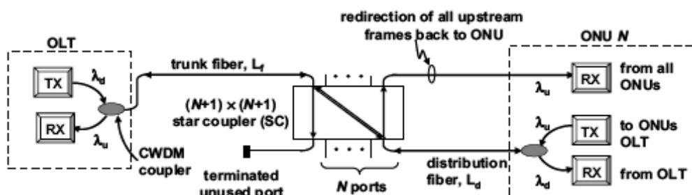
Figure 20. Physical Architecture of EPON
