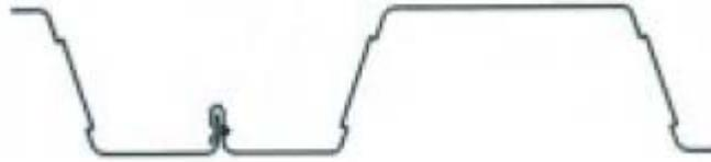
*Fig 1.13: Fold on the connection of two sheets (seam connection) Extracted from [9]*
