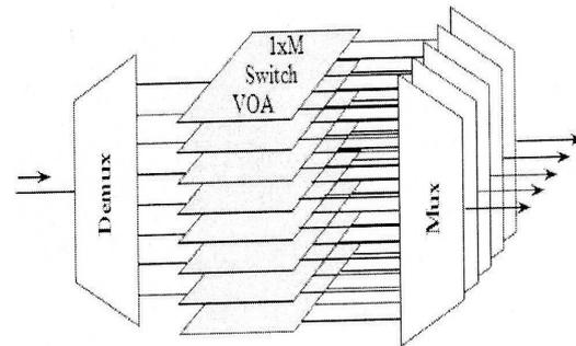
Figure 5: Model of a WSS for simulation
