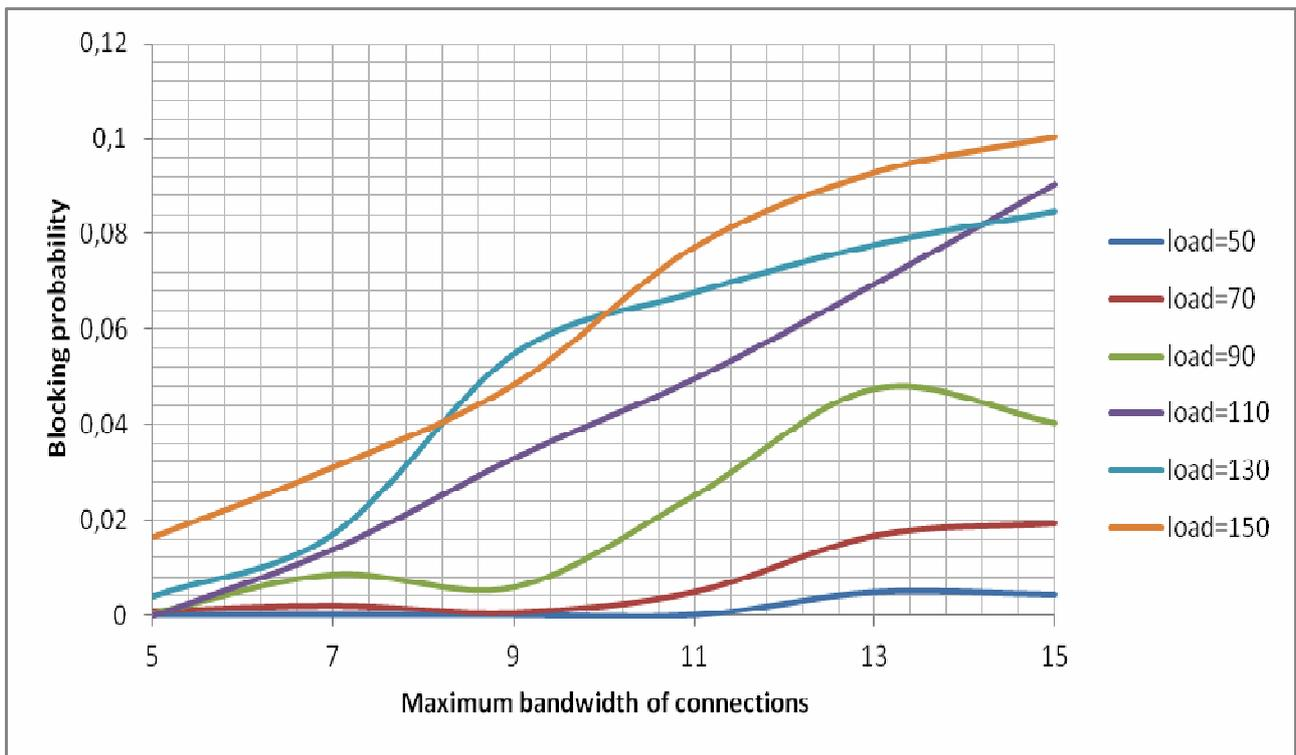
Figure 11: Blocking probability of the designed node depending on the maximum bandwidth and the traffic load
