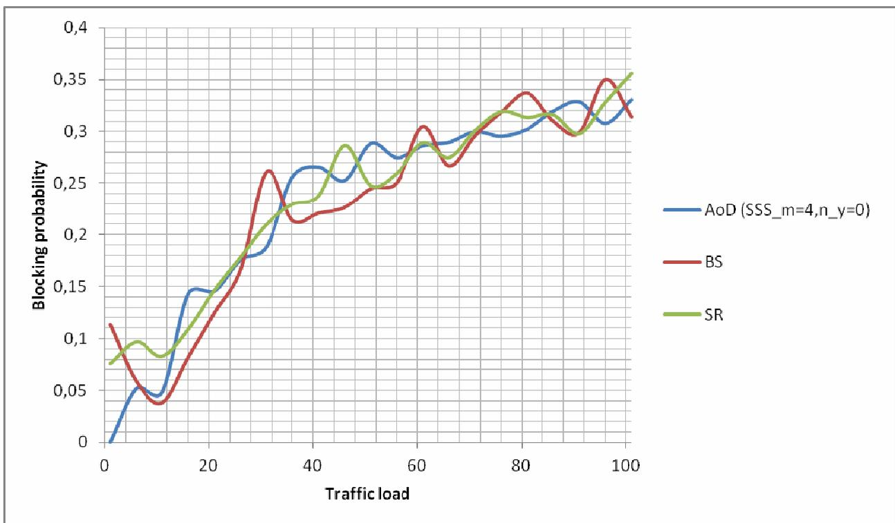
Figure 6: Comparison of the three architectures, with AoD without wavelength converters
