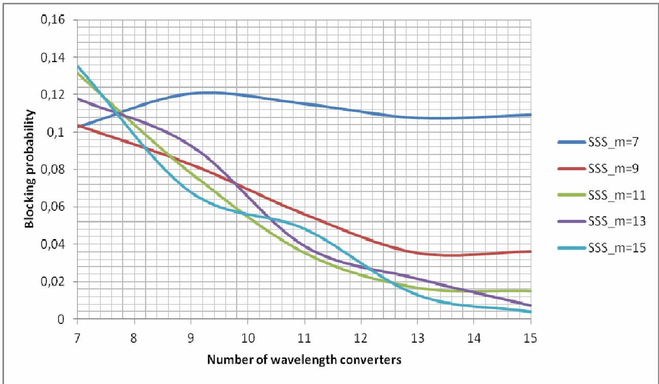
Figure 7: Blocking probability depending on the number of wavelength converters, for different amount of SSS modules' ports
