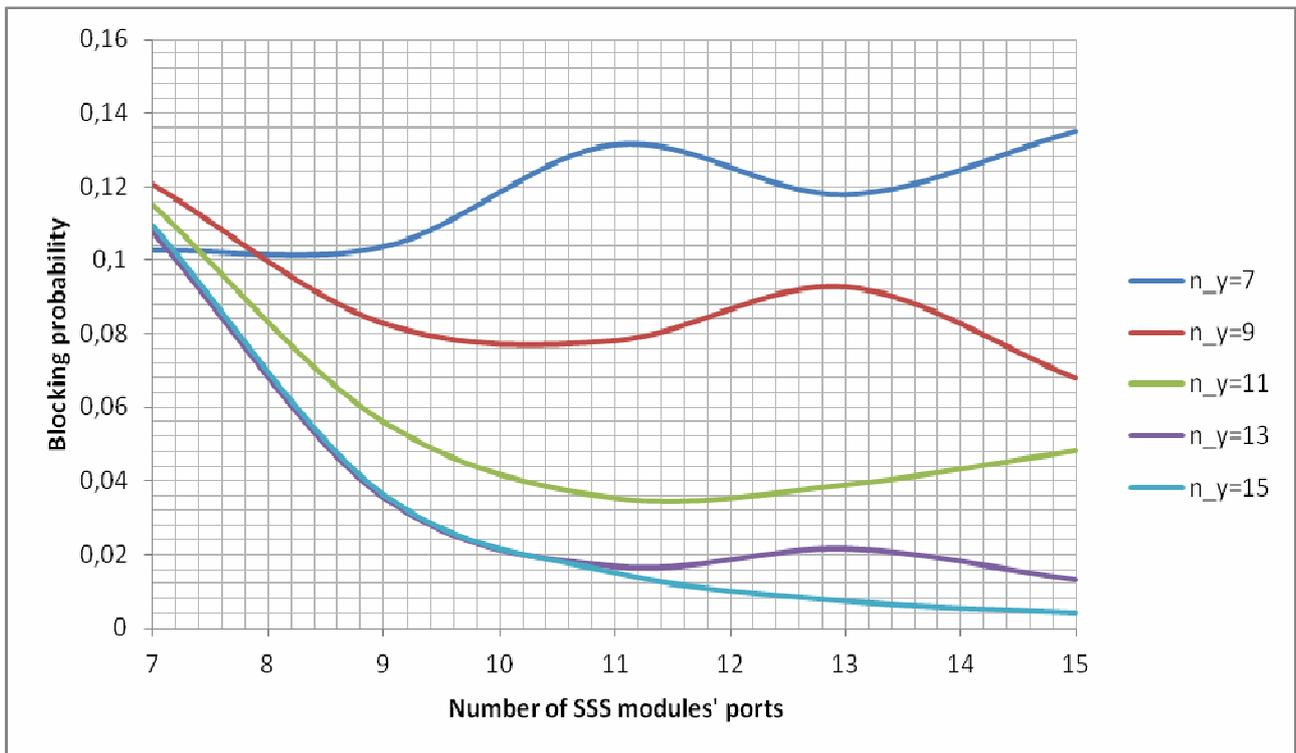
Figure 8: Blocking probability depending on the number of SSS modules' ports, for different amount of wavelength converters
