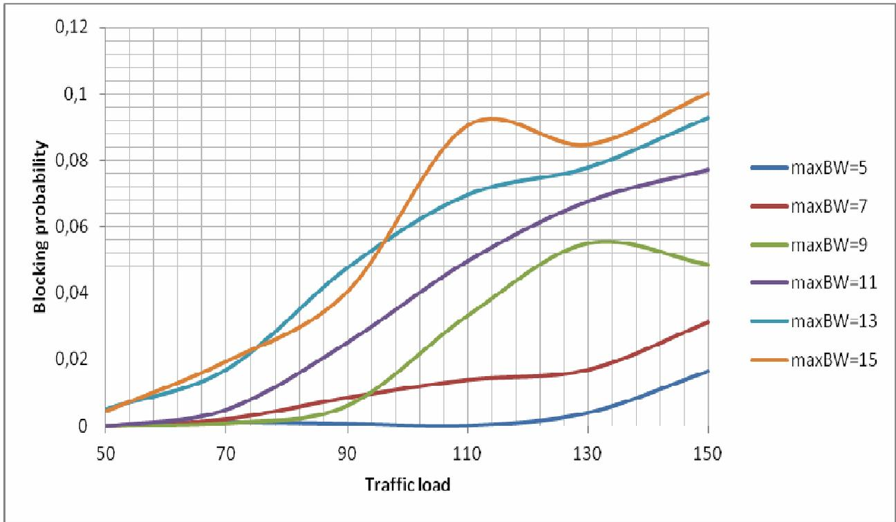
Figure 10: Blocking probability of the designed node depending on the traffic load and maximum bandwidth
