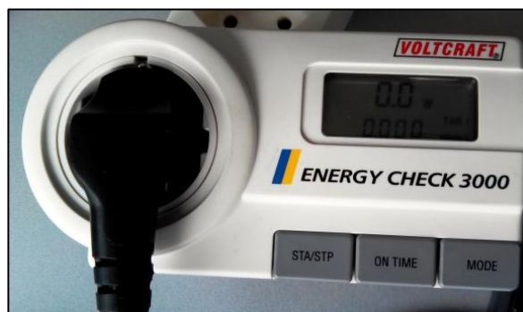
Figure 8.4 – Commercial power meter.
