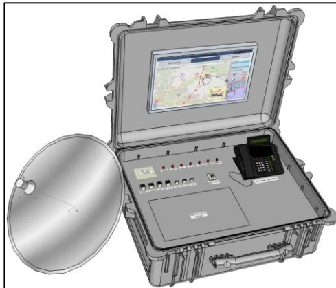
Figure 3.3 –3D sketch of a PLMU based on a Pelican 1600 case [5].
