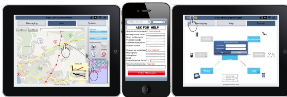
Figure 5.3 GUI mock-ups, from left to right: First responders' GUI, victim's GUI and technicians' GUI
