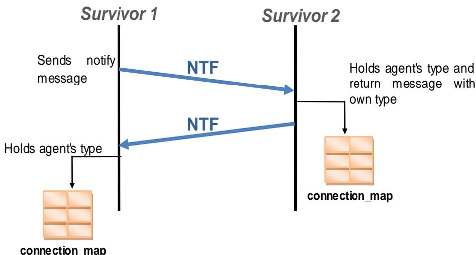
Figure III.8 Diagram of the messages transaction involved into the Start-up Protocol
