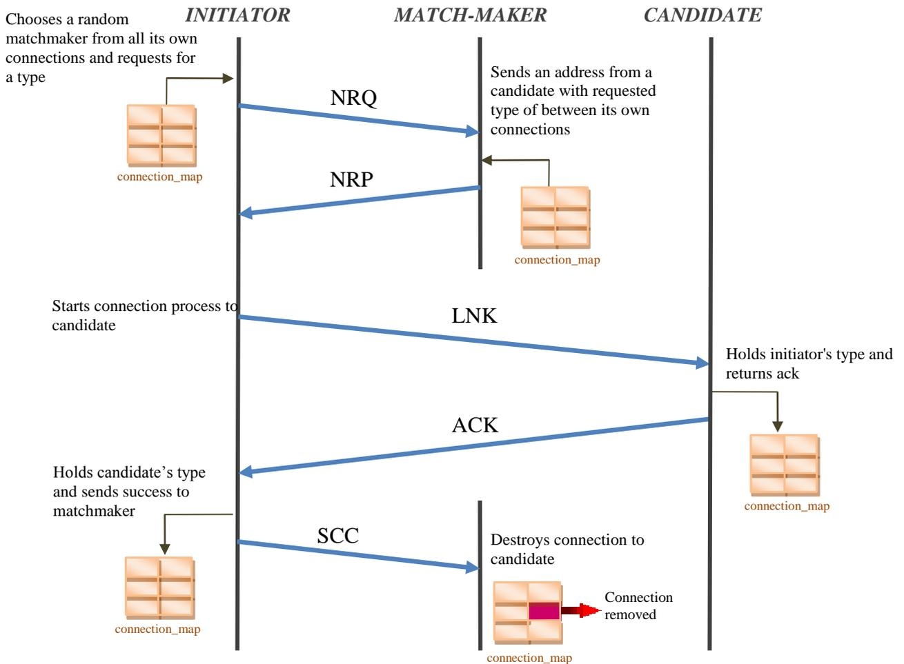
Figure III.11 Diagram of the messages transaction involved into the Aggregation Protocol
