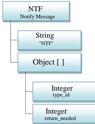
*Figure III.10 Structure of the Notify Message*
