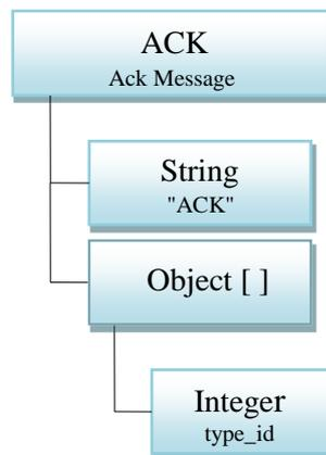
*Figure III.16 Structure of the Ack Message*
