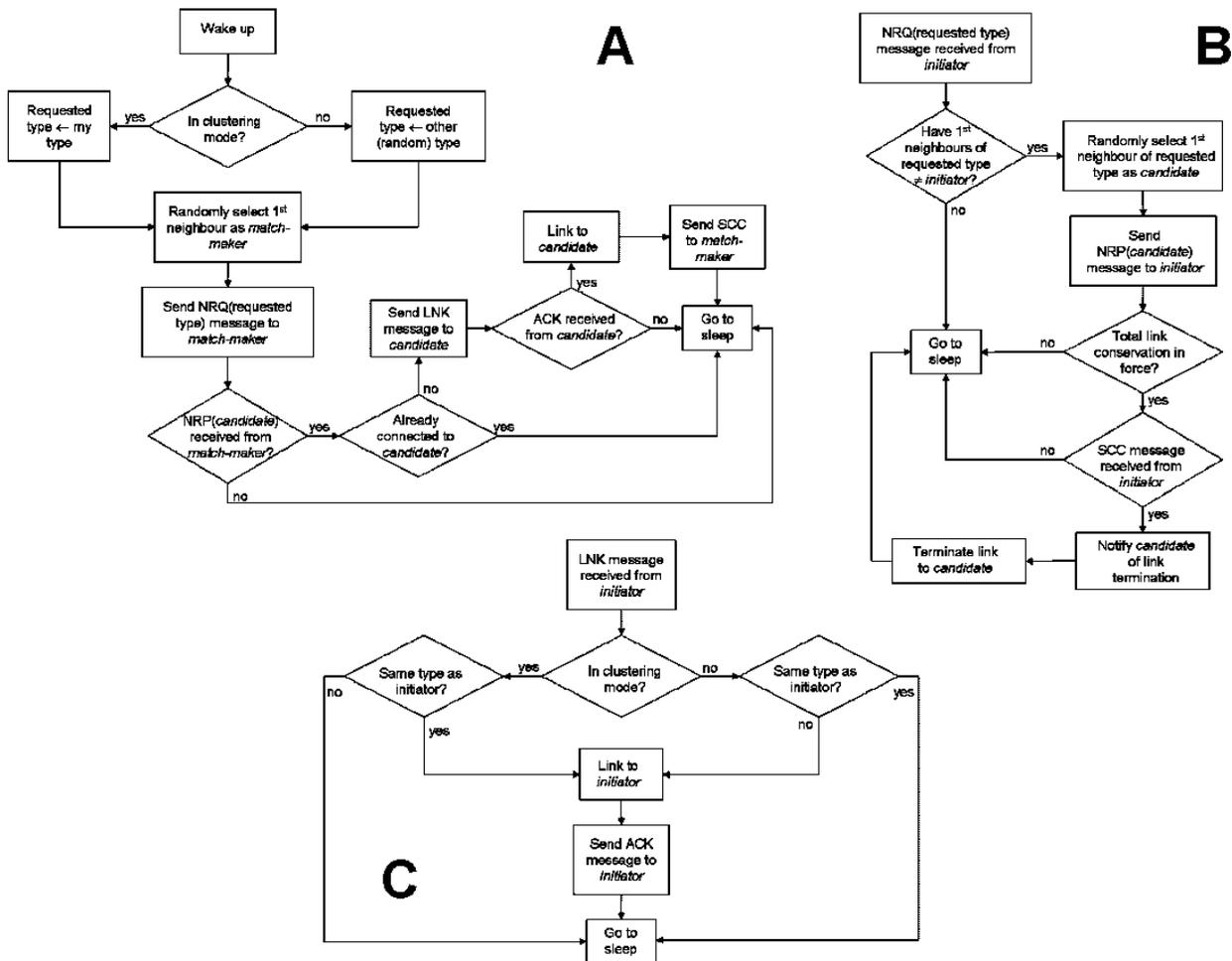
Figure II.5 Algorithms involved in rewiring operation following the “on-demand” clustering procedure with the three roles of “initiator”, “match-maker” and “candidate”.
