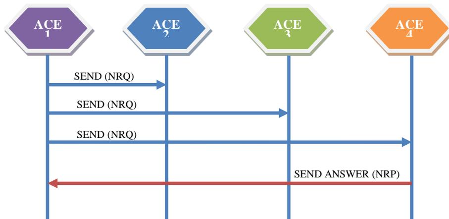
Figure III.12 Requests Messages are re-send by the initiator agent to the different match-makers chosen till receive an answer
