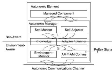
Figure 1 – Example of an Autonomic Element
