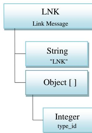
Figure III.15 Structure of the Link Message
