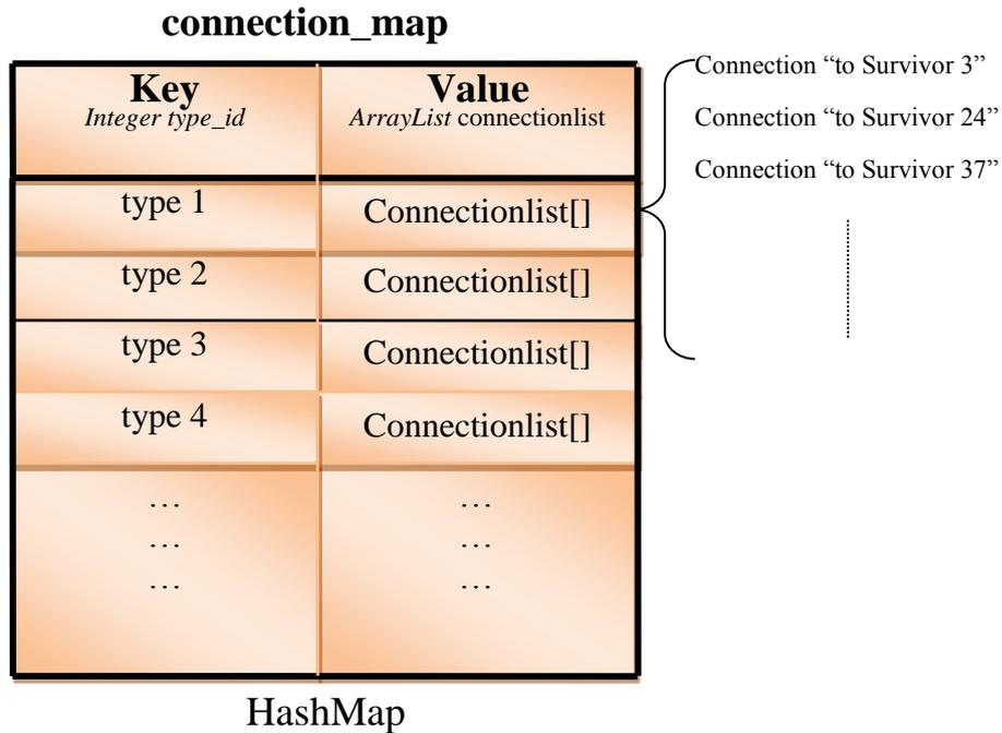
*Figure III.9 Structure of the HashMap in charge of storing all connections discovered mapping them according to their type*
