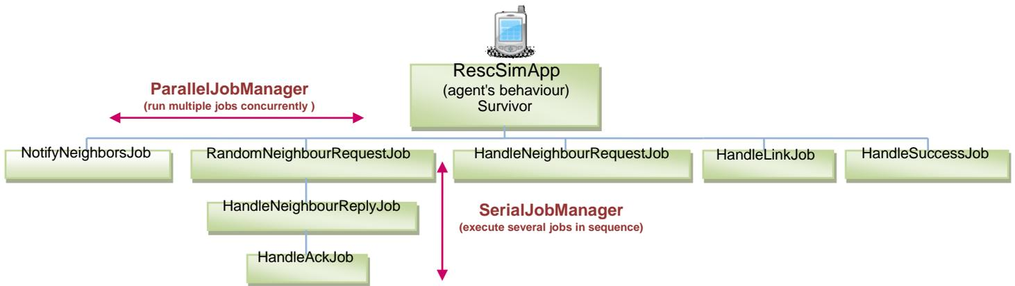
Figure III.18 Jobs' Structure working managed by the ParallelJobManager and the SerialJobManager which compose the Agent's behaviour
