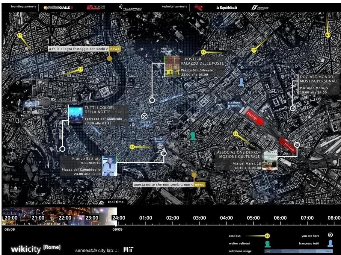
Figure II.8 Real Time Rome project using cell phones and GPS devices to collect the movement patterns of people and transportation systems
