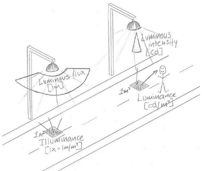
Luminous flux, illuminance, luminous intensity and luminance are all taken into consideration and used as properties for investigating the quality of the light. Briefly, summarized it is found that the LED lighting in the position intended will supply sufficient lighting on the street while not polluting the skies with excessive lighting.
