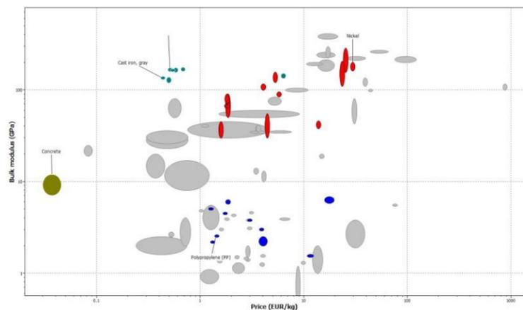
As seen on the picture concrete (read: brown circle) is here the most optimal solution in regards to price and bulk modulus.
