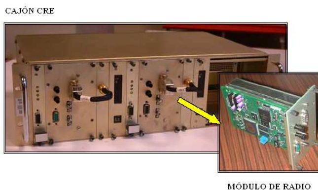
Fig. 161 Cajón del Carbonne Radio Equipment (CRE).
