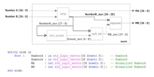
The code could be divided in two parts. The first one implements the connection between the different blocks which the mixed numbers entity works with. The block diagram is coherent with the VHDL code.
