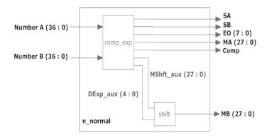
Figure 18. Normal numbers block diagram
