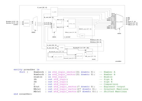
The components description is shown in this part of the code. Normal numbers block ( $n\_normal$ ), subnormal numbers block ( $n\_subn$ ), mixed numbers block (*norm*), the multiplexor and demultiplexors ( $mux\_ns$ ,  $mux\_adder$  and demux) and the *selector* entity are added there.
