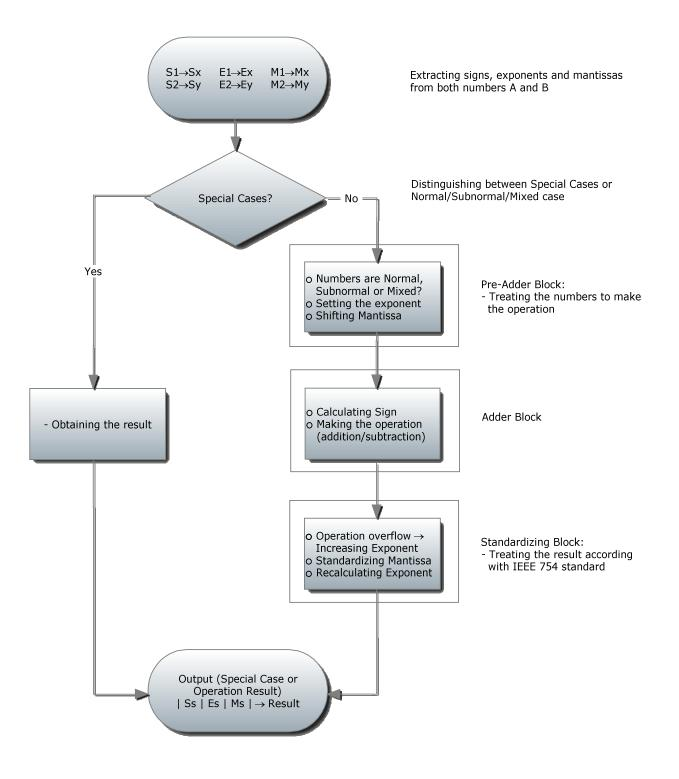
Figure 6. Block Diagram Code
