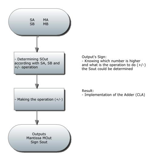
Figure 8. Adder Block Diagram
