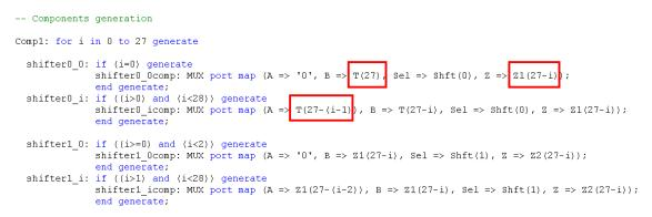
Changing the order of the vector, a displacement in the other direction is achieved. The simulation is not required because the result is the same but on the right.
