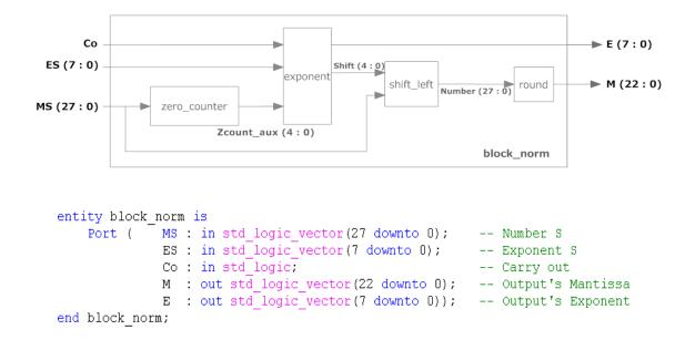
The first part of the code implements the connection between the different components which compose the block. *Zero, shift\_left* and *round* are connected as shown in the code and the block diagram.
