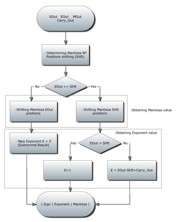
Figure 9. Standardizing Block Diagram
