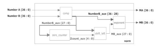
Figure 12. Mixed numbers block diagram
