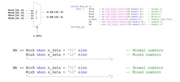
Finally *mux\_adder* multiplexor is in charge of selecting which data are going to be introduced in the adder.
