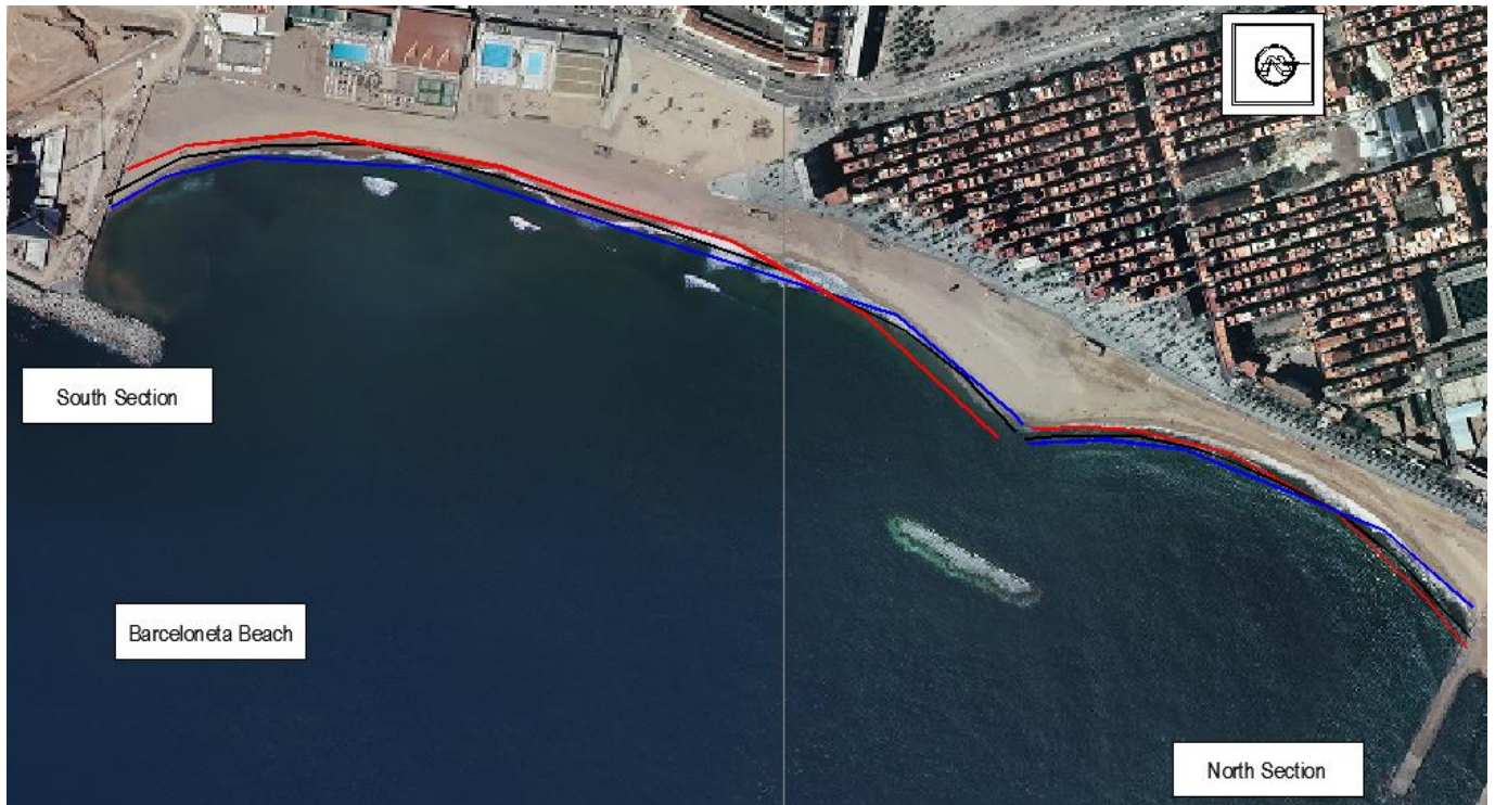
Figure 66 Theoretical Model of Barceloneta after 2006 (Photo: Ortophotos 2008, ICC) North Section : Configuration 1, shoreline of December 30, 2008 (solid blue line), Configuration 2, shoreline of December 31, 2009 (solid black line) and Configuration 3, shoreline June 23, 2009 (solid red line). South Section : Configuration 1, shoreline of November 15, 2007 (solid blue line), Configuration 2, shoreline of June 23, 2009 (solid black line) and Configuration 3, shoreline April 14, 2009 (solid red line).
