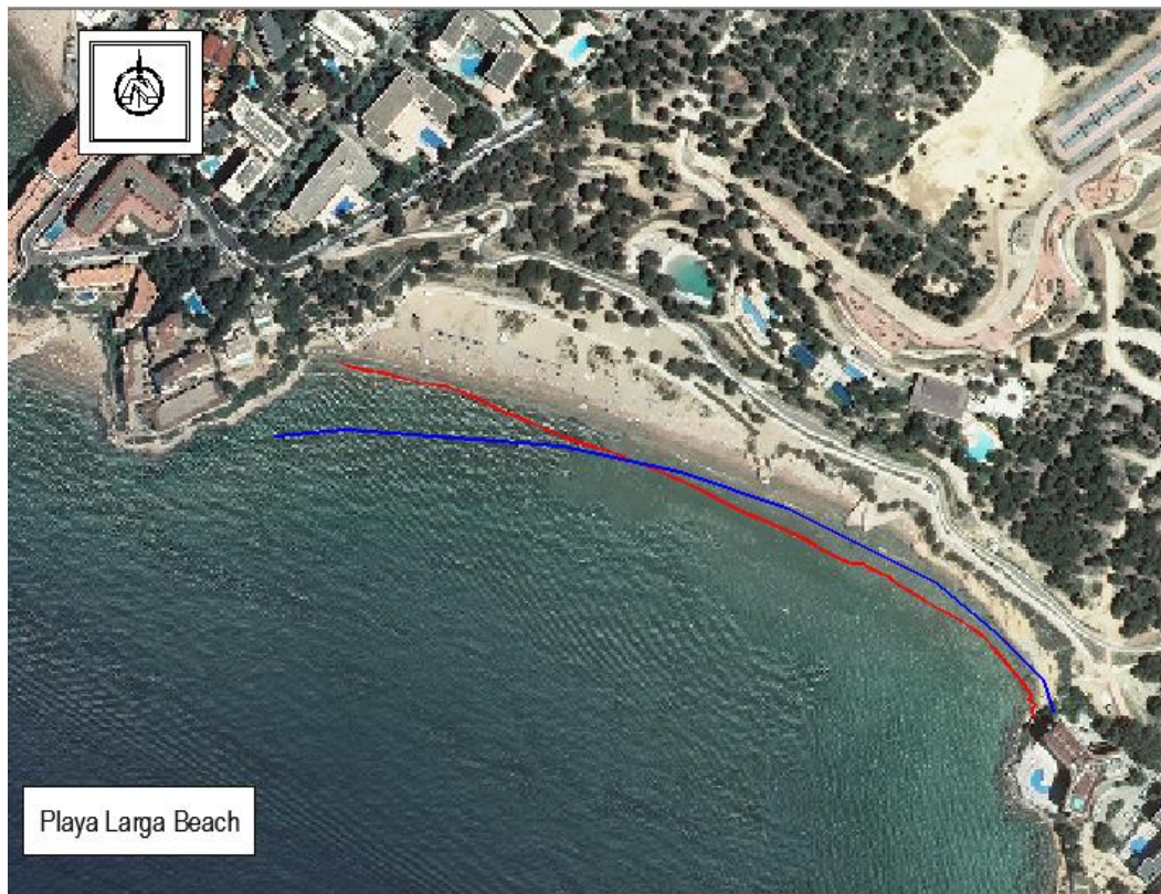
Figure 73 Theoretical Model of Playa Larga (Photo: Ortophotos 2008, ICC) Configuration 1, shoreline of November 11, 2007 (solid blue line), Configuration 2, shoreline of March 1 st , 1995(solid red line).
