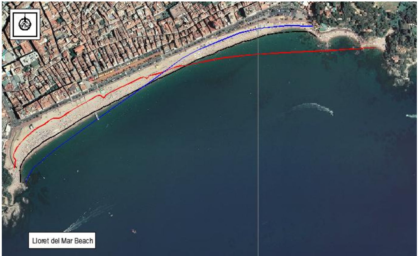
Figure 42 Theoretical Model of Lloret del Mar (Photo: Ortophotos 2008, ICC). Configuration 1, shoreline of April 27, 2004 (solid blue line), Configuration 2, shoreline of July 1 st , 1986 (solid black line) and Configuration 3, shoreline May 1 st , 2001 (solid red line).
