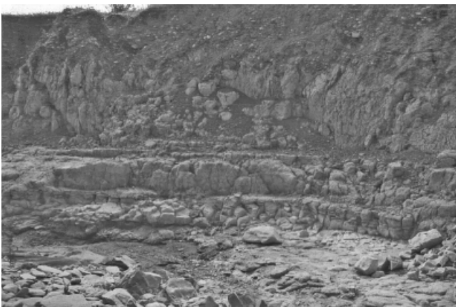
Fig. 8. Exposed outcrops of Guadalquivir clay showing horizontal bedding planes: river banks of Agrio river
