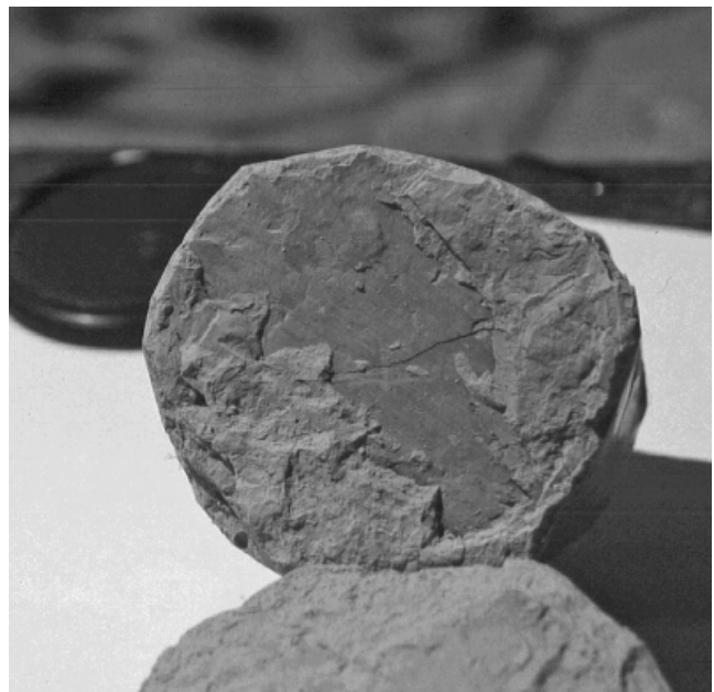
Fig. 10. Slickensides observed in core recovered in borehole S1-3 at 13.5 m depth
