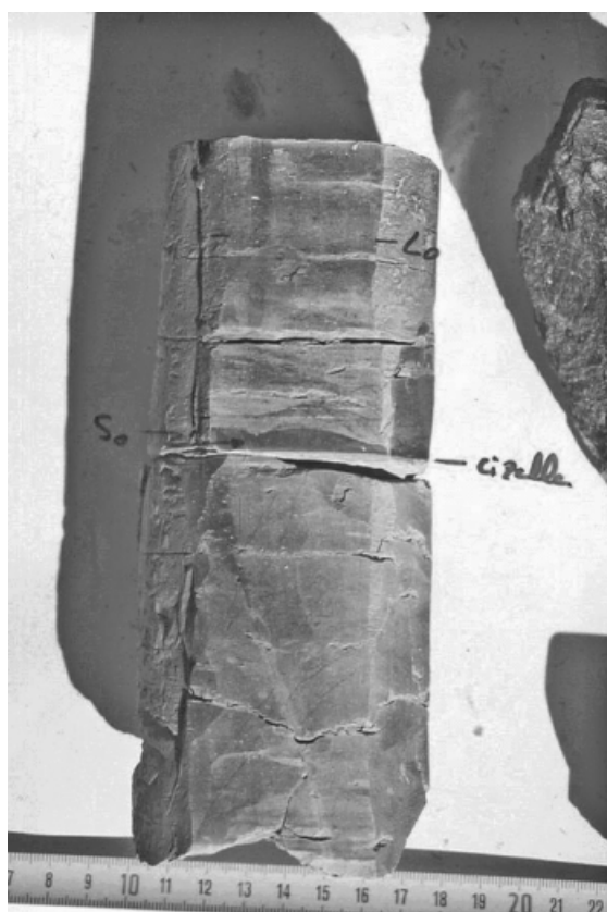
Fig. 18. Highly polished and striated shear plane that follows a bedding plane ( S_0 ). Borehole 2-1 at 33.8 m depth. It was interpreted as belonging to the sliding surface
