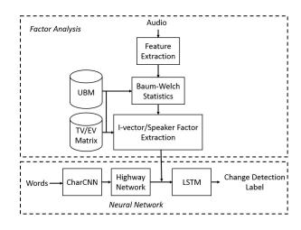
Figure 1: System architecture
